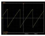
Figure 1 An Incremental Counter Signal
